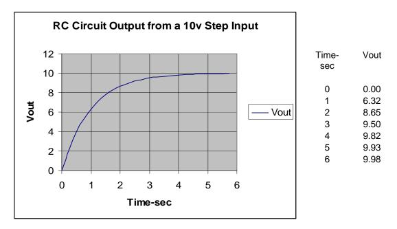
One should see that in 1 Time Constant (1TC) the output reaches about 63% of full value and that after 5T (five Time Constants which is 5 seconds in our case) the output reaches 99% of the full 10v input.
