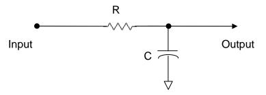
It turns out that in this configuration, should one suddenly place a step function on the input, the output voltage would rise to meet the input following the equation as shown below.
