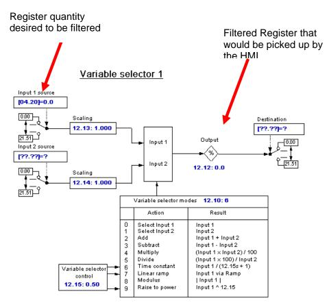
Note that the Output register #12.12 and #12.32 will be 100% at the full value of the input register. For instance, in this example #4.20 (% Load ) is %Load of the motor which could be 165% possibly. Hence, the output register will be 100% at this value- the HMI displayed register would need to be scaled accordingly.
