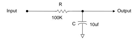
The larger value of RC, the longer the time constant. If this RC circuit consisted of a 100K resistor and 10uf capacitor, the time constant would be:
