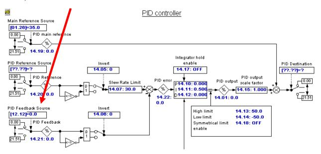
For Pressure, Level or Temperature Control systems, feedback is usually rather slow and filtering time constants of 0.5 - 1 seconds may be tolerable.
