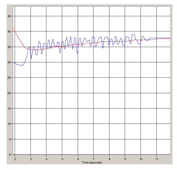
To filter noisy temperature or pressure transducer signals a Time Constant this large may be ok.
